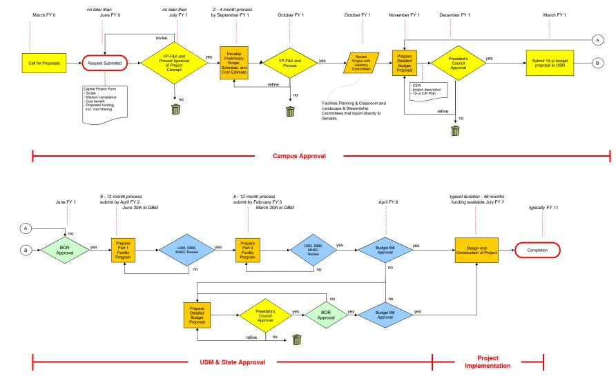
Figure 2: Flowchart outlining the approval, planning, and implementation process for major facilities projects at UMBC funded through the State's Capital Improvement Program.
